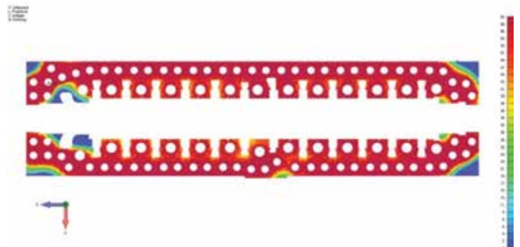
Fig 1. Result of FEA of packing under a test pressure of 276 bar. No leaking was found.
